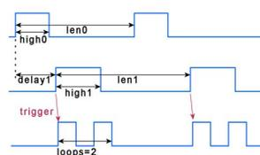
The digital pulse generator option adds 4 internal independent digital pulse generators with programmable duty cycle, output frequency, delay and number of loops. These digital pulse generators can be triggered by software, hardware trigger or can trigger each other allowing to form complex pulse schemes to drive external equipment or experiments. The digital pulse generators can
